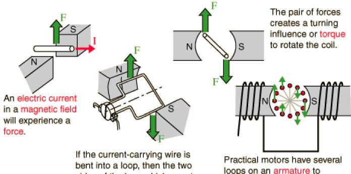
If the current-carrying wire is bent into a loop, then the two sides of the loop which are at right angles to the magnetic field will experience forces in opposite directions.
