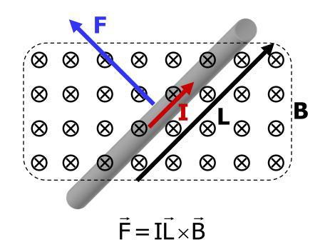
Valid for straight wire, length L inside region of magnetic field, constant magnetic field, constant current I, direction of L is direction of conventional current I.
