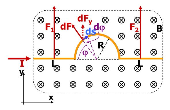
Does symmetry give you  $F_x$ immediately? Or, you can calculate the x component of F.  $dF_x = -I R d\phi B cos\phi$
