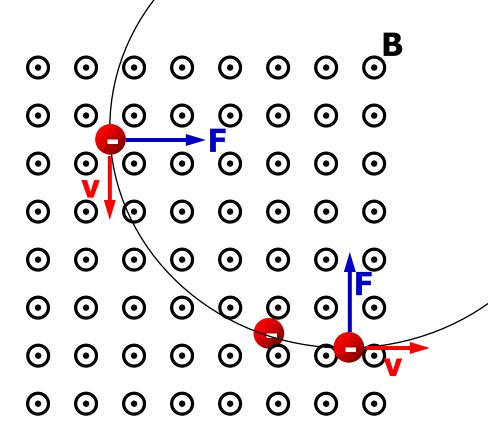
The electron will move in a circular path with an acceleration equal to  $v^2/r$ , where r is the radius of the circle. Pradeep Singla
