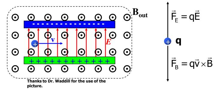
When the electric and magnetic forces balance then the charge will pass straight through. This occurs when  $F_E$ =  $F_B$  or qE = qvB or  $v = \frac{E}{r}$
