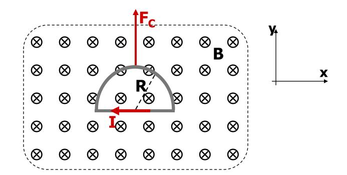
We calculated the force on the semicircular part in the previous example (current is flowing in the same direction there as before) = 2 IRB
