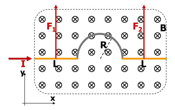
Next look at the  $\otimes$ semicircular  $\otimes$ section. **Calculate the**  $\otimes$ incremental force  $\otimes$ dF on an incremental ds of (X)current-carrying wire. ds subtends the angle from  $\varphi$  to **φ+dφ.** The incremental force  $id\vec{F} = I d\vec{s} \times \vec{B}$ .
