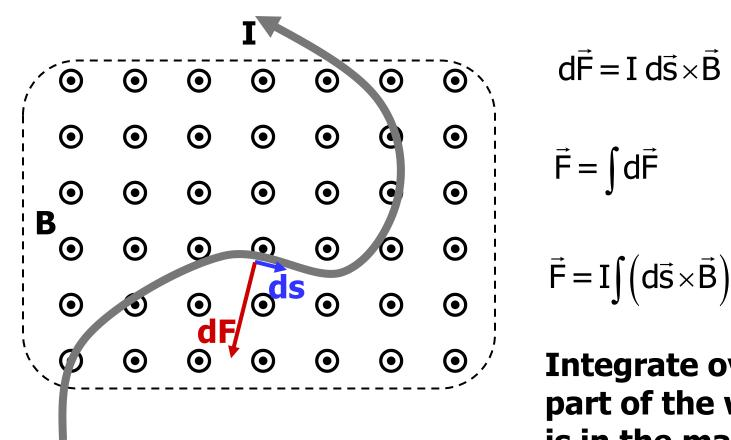
Integrate over the part of the wire that is in the magnetic field region. Example: a wire carrying current I consists of a semicircle of radius R and two horizontal straight portions each of length L. It is in a region of constant magnetic field as shown. What is the net magnetic
