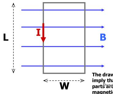
Let the loop carry a counterclockwise current I and have length L and width W.
